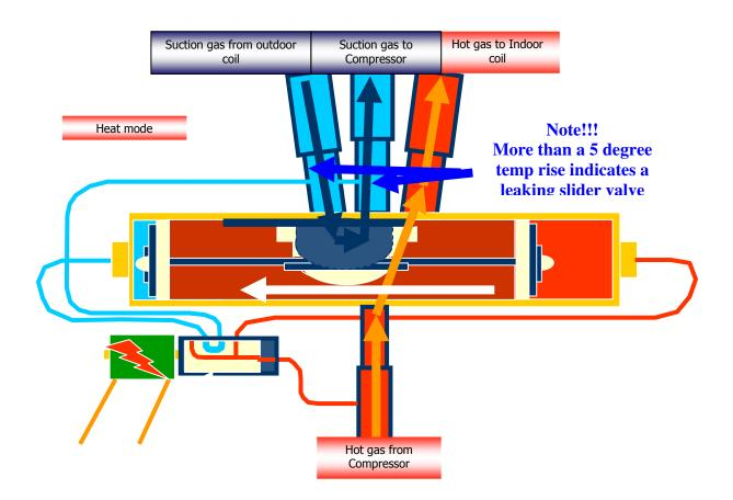
If a system is low on charge the pressure from the hot gas line is lowered, this could cause the reversing valve to not fully shift.
