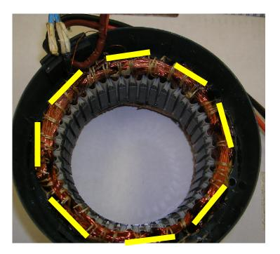
It is now easy to count the poles (8) and compare it to the chart above to determine a PSC motor rpm (825). Give it a try sometime.
