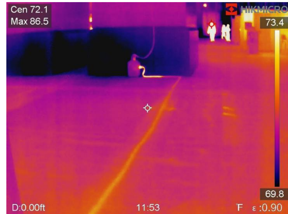
Warm electrical cord conducting heat to the carpet
