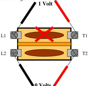
No measureable voltage should be read across the energized terminals of a switch or fuse unless it is open.
