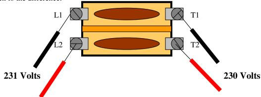
The proper way to check is to measure *across the contacts* <u>as well</u>. Any voltage reading of 1 or more volts indicates the contacts are not properly closing and should be <u>recommended to be replaced</u>. This 1 volt drop tells the technician that the switch has become a load and <u>will produce heat</u>. This will continue to heat up dropping more voltage until either it burns up the contacts or robs enough voltage from the compressor to possibly cause damage to it as well.
