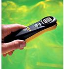
After zeroing the meter outdoors, remove the CO 205 aspirator from the CO 220 detector. Walk through the home taking readings on various levels. A home with smokers in it or a customer that burns candles may have readings of 1-3ppm in the home. While EPA sets the maximum of 9ppm over 24 hours, testing has shown that levels of 5 ppm or greater should be investigated.
