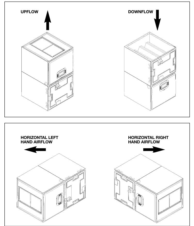
**NOTE:** Coil and blower section are always in a draw through configuration.
