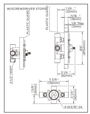
Critical Dimensions: Rough-in valve GS-314-PK (w/stops) & GS-317-PK (w/stops)
