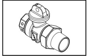
**5/8" VALVE WITH FLARE COPPER INLET BY FEMALE IRON PIPE THREAD OUTLET**
