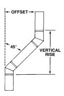
**Note:** The vertical rise can also be closely estimated by adding one "A" and one "B" dimension to Maximum Offset figures. (See dimensions of Round Adjustable 45° Elbows.)
