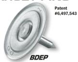
Target (BDEP) pins are a patented insulation fastener designed with an aerodynamic embossed washer and a recessed nail head to improve the quilting contour of the secured duct liner.
