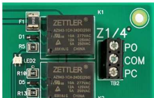
Zone panel damper connection terminals
