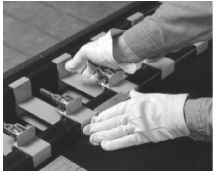
10. Duct board grooving machine set up for cutting ten-sided fibrous glass duct.
