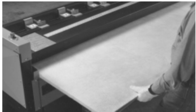
#5 (or G). Right hand square cut tool with closure flap.
