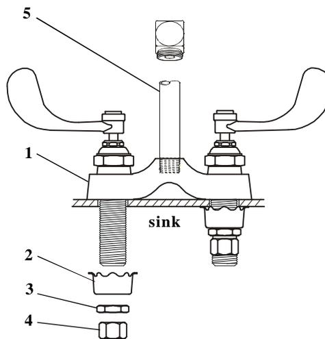
3. Place no. 1 into holes in sink top and replace no. 2, no. 3 and no. 4 onto threaded shank. Tighten no. 4 firmly with a wrench.
