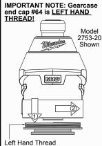
As an aid to assembly, carefully lower the complete front end of tool (gearcase/impacting system) onto the gearcase end cap. Gently hand tighten front end assembly onto gearcase end cap. Be careful not to cross-thread! Once installed by hand, seat gearcase end cap with a good adjustable wrench using light pressure.
