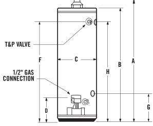
Maximum Hydrostatic Working Pressure: 150 PSI
