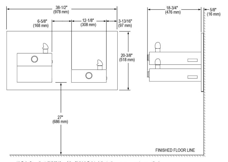
\*A.D.A. Compliant (24" [610mm] for Child A.D.A.). Adjust other measurements accordingly EHWM17C shown with accessory apron LKAPR2 mounted.
