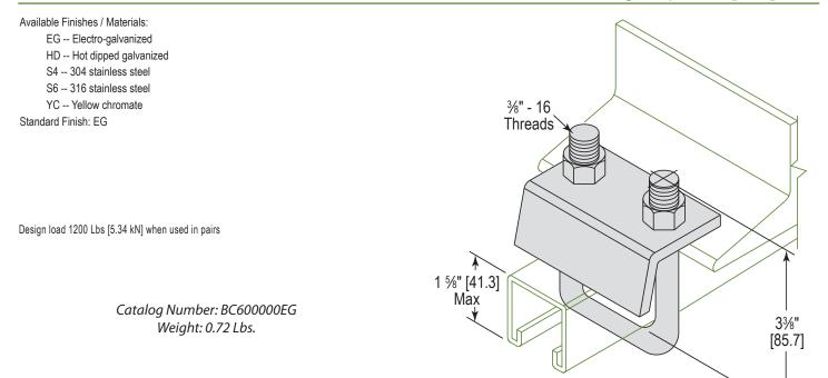
Material is 1<sup>5</sup>/<sup>6</sup>" [41.3] wide x <sup>1</sup>/<sub>4</sub>" [6.3] thick unless specified. Holes are <sup>5</sup>/<sub>6</sub>" (14.3) diameter, <sup>1</sup>/<sub>6</sub>" [20.6] center to edge on 1<sup>7</sup>/<sub>6</sub>" [47.6] centers unless specified.
