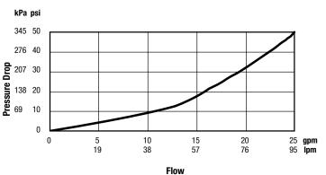
Flow curves are for reference. Actual flows may vary depending on system temperatures and/or pressures. \*Flow curve with integral inlet filters check valves
