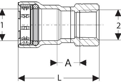
MegaPress Adapter, Carbon Steel, P x FPT - Models 4812 / 6612
