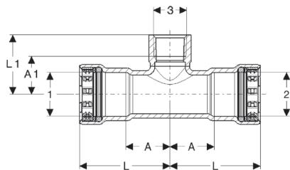
MegaPress Reducing Tee, Carbon Steel, P x P x FPT - Models 4817.2 / 6617.2
