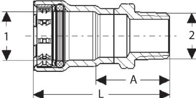
MegaPress Adapter, Carbon Steel, P x MPT - Models 4811 / 6611
