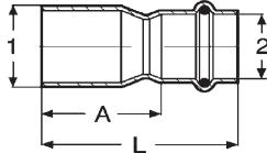
Viega ProPress Reducer Copper FTG x P - Model 2915.1
