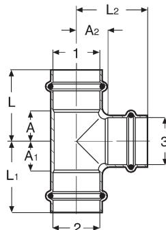
Viega ProPress Tee Copper P x P x P - Model 2918
