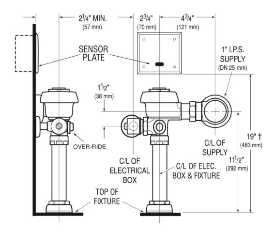
† Position of Sensor Box can be raised or lowered 1" (25 mm) if in conflict with Handicap Grab Bars.
