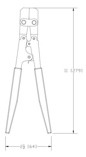
**Engineering Specification:** Zurn Stainless Steel Crimp Ring Tool. The QSECRT is a calibrated tool conforming to ASTM F2098 that applies the recommended force needed to make a leak-free crimp connection. The SSC tool is used with the stainless steel crimp rings, the Qick/Sert1<sup>®</sup> or QickSert CR<sup>TM</sup> fittings, and ZurnPEX<sup>®</sup> tubing to make a leak-free plumbing system.
