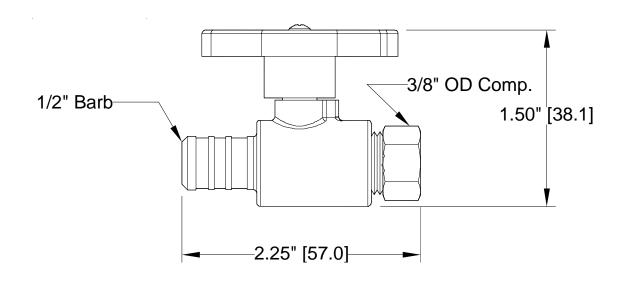
**Engineering Specification**: Zurn PEX<sup>®</sup> XL-Low Lead Brass Quarter-Turn Straight Stop Valve. The QQTV60SGX has a 1/2" PEX barb inlet x 3/8" 0.D. compression outlet. Manufactured from EcoBrass<sup>®</sup>,C69300. These fittings, as a system with Zurn PEX<sup>®</sup> tube, are pressure rated at 160 PSI at 73°F, 100 PSI at 180°F, and 80 PSI at 200°F. These fittings are listed as complying with the following standards: NSF/ANSI Standard 61 including Annex G, CSA B137.5, and ASTM F1807.
