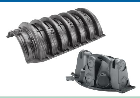
The evolutionary patent-pending Quick4® Standard Chamber fits in a 36" wide trench and is ideal for curved or straight systems. It features the patent-pending Contour Swivel Connection™ which permits 10-degree turns, right or left. The MultiPort™ end cap allows multiple piping options and eliminates pipe fittings. The chamber's four-foot length provides optimal installation flexibility.
