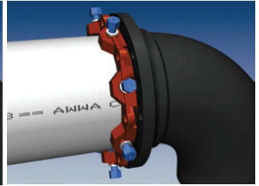
1. Identify the pipe. The 2000PV is for use with PVC and HDPE pipe. The 4 inch through 12 inch size may be used on C900, IPS, and C909 PVC pipe as well as C906 HDPE pipe. Check to see if the spacers under the screws are in place. If the pipe is C900 or is ductile iron O.D., proceed with spacers in place. If the pipe is IPS O.D., remove the spacers. Since 3 inch and 14 inch through 24 inch restraints are only used with one pipe diameter, no spacers are used.
