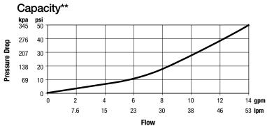
Flow curves are for reference. Actual flows may vary depending on system temperatures and/or pressures. \*\*Flow curve with integral inlet filters and check valves
