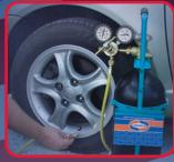
Inflate tire with the Sludge Sucker® Air Chuck
