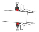
ONE-LOK's carn action also accommodates deflection of the joint during installation, and also allows for subsidence, seismic or other forces after installation, up to the maximum allowed deflection.
