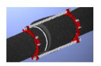
3. Insert the threaded rods provided and snug the retaining nuts against the restrainer ears (against the flat surface). Do not overtighten retaining nuts, approximately one turn with a wrench.
