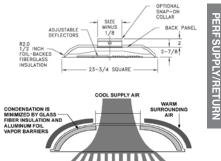
COOL SUPPLY AIR IS DIFFUSED ALONG CEILING SURFACE THE COOL AIR MIXES WITH ROOM AIR AND FILTERS DOWN
