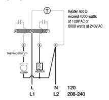
Models 8041-00 and 8041-20 - Wiring Diagram
