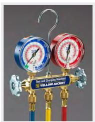
Series 41 manifolds are also available with larger, easier to read 3-1/8" color-coded gauges in rugged steel cases with polycarbonate crystals. These gauges feature 1% accuracy (Class 1) for an exact reading in critical charge systems.
