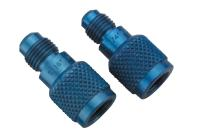
Liquid charging is recommended when charging blends into refrigeration and air conditioning systems. A liquid charging adapter is necessary for safe and fast liquid (saturated vapor) charging through the low pressure side of a system. The YELLOW JACKET liquid charging adapter connects to the cylinder valve or refrigerant tank.
