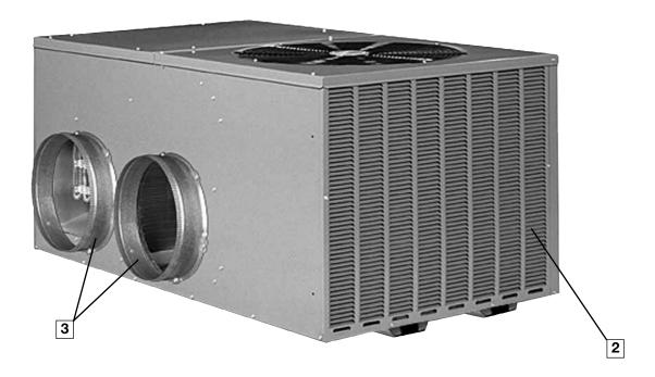
To provide flexibility in space-limited installations, the unit can be installed flush to the structure without blocking airflow over the outdoor coil or making any screws inaccessible for maintenance. Furthermore, the cabinet is a slim 33" wide. Full-louver coil protection (2) makes Ruud unique in the industry and also totally protects the outdoor coil from vandalism and weather extremes.
