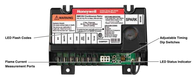
Suitable for use with or without vent dampers the S8610U provides the ignition sequence, flame monitoring and 100 percent safety shutoff for intermittent pilot central furnaces and heating appliances. Enhancements that improve the performance and simplify troubleshooting highlight the latest release of the Universal control.
