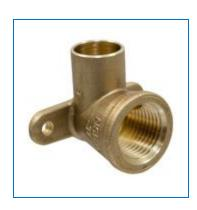
**Specifications UPC** Code 039923299826 All Type of Item **Fitting All Special Application** Lead-Free\* **Description** 707-3-5-LF 1 CXF 90 DROP ELB CAST **Fitting Bend Angle** 90 Deg (1/4 Bend) Elbow **Type Connection Type** C x F (NPT) 0.485 lb Weight Size 1 Material Lead-Free Bronze
