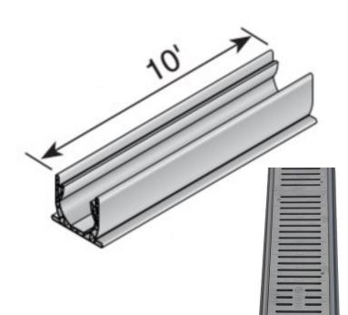
Part #: 400 –10WH Channel Material: PVC Grate Material: HDPE Color: Channel Gray Grate: Gray UV Inhibitors Weight: 17.5 lbs Grate opening: 1/4" x 3-1/8"" Open Surface Area: 16.92 sq. in. per ft. Flow Capacity: 103.49 GPM with 0.5" head 146.36 GPM with 1" head
