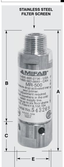
**Specification:** MIFAB® model MR-500-NPB pressure drop activated brass trap seal primer, with inlet opening of  $\frac{1}{2}$ " (13) male N.P.T. and outlet opening of female  $\frac{1}{2}$ " (13) N.P.T. Complete with four view holes and removable filter screen. Serves up to 6 floor drain traps and requires no adjustments and no air pre-charge.
