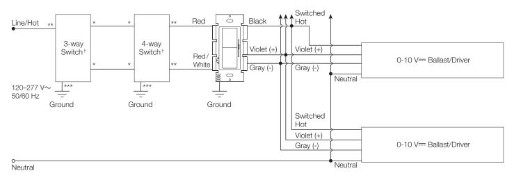
Note: For 4-way wiring, control must be installed line side or load side. It cannot be installed in the 4-way location.
