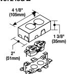
15A, 125V Duplex Grounding Receptacle (Nema 5-15R) and Box – Accommodates other standard 15A (NEMA 5-15R) or 20A (NEMA 5-20R) duplex devices in place of furnished duplex grounding receptacle. Cover has twistouts for V500 and V700 on each end and side. End twistouts permit running raceway close to interior trim. Base has 1/2" trade size KOs.
