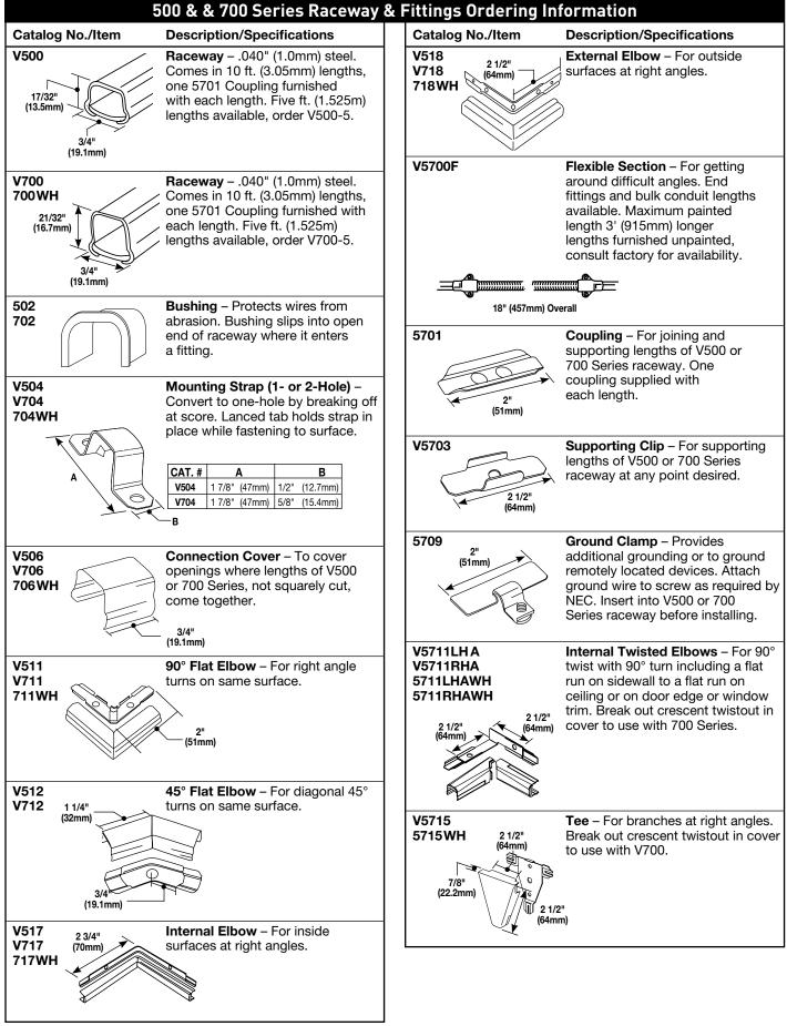
NOTE: Use #6 flat head screws with all fittings requiring screws except V504/V704, and V57200 Series; with V504/V704 use #8 pan head screws; with V57200 Series use #8 flat head screws.
