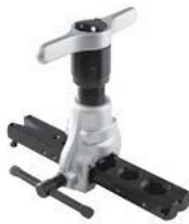
T30600 Ratcheting, eccentric cone flaring tool with internal clutch to prevent over-torquing. For tube OD: 3/16", 1/4", 5/16", 3/8", 1/2", 5/8" and 3/4"
