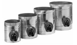
The TrueZONE<sup>®</sup> Bypass constant pressure regulating damper (CPRD) is a round static pressure relief damper. It is used in forced-air bypass applications to relieve excess static pressure when some of the zone dampers are closed.
