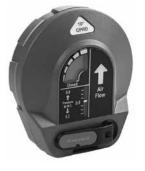
The TrueZONE<sup>®</sup> Bypass constant pressure regulating damper (CPRD) is a round static pressure relief damper. It is used in forced-air bypass applications to relieve excess static pressure when some of the zone dampers are closed.
