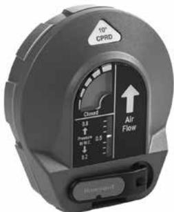
The TrueZONE® Bypass constant pressure regulating damper (CPRD) is a round static pressure relief damper. It is used in forced-air bypass applications to relieve excess static pressure when some of the zone dampers are closed.
