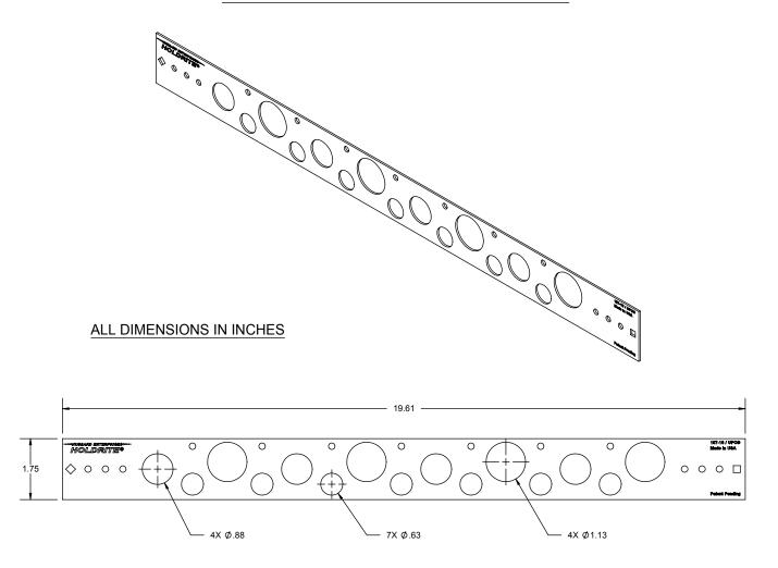
The HOLDRITE #107-18 is a Copper-Bonded™ steel bracket with holes on 2" centers to position 1/2" copper tubing and holes on 4" centers to position 3/4" and 1" copper tubing.
