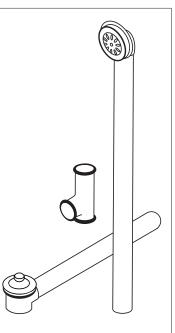
Attach the waste and overflow tee (D) to the overflow assembly (C) and shoe assembly (A) with sealing washers and slip nuts.
