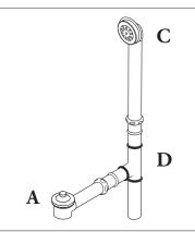
Attach the drain tube and flange (E) to the waste and overflow tee (D) with the sealing washer and slip nut.
