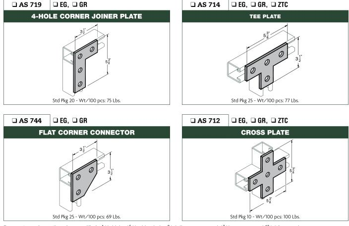
Page notes unless otherwise specified: 1/4" thick, 15%" wide, holes 9/16" diameter, spaced 17/8" on center and 13/16" from end.
