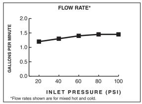
1.5gpm/5.7 L/min. FLOW RATE
