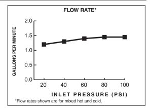
1.5 gpm/5.7 L/min. FLOW RATE
