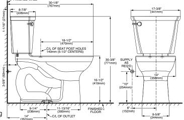
NOTES: THIS TOILET IS DESIGNED TO ROUGH-IN AT A MINIMUM DIMENSION OF 356MM (14") FROM FINISHED WALL TO C/L OF OUTLET.
